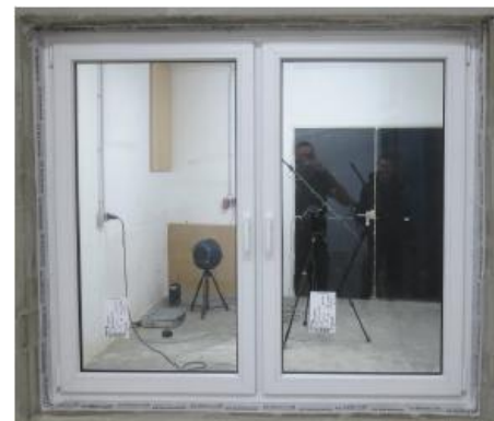
Figure 4: View of the reference window with closed casements, installed in the test laboratory.
